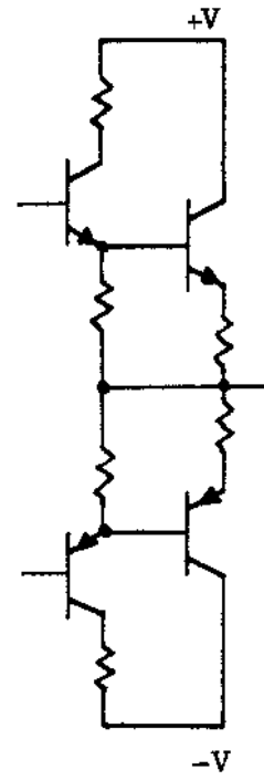
Fig. 2. True complementary circuit used by JBL and Accuphase
