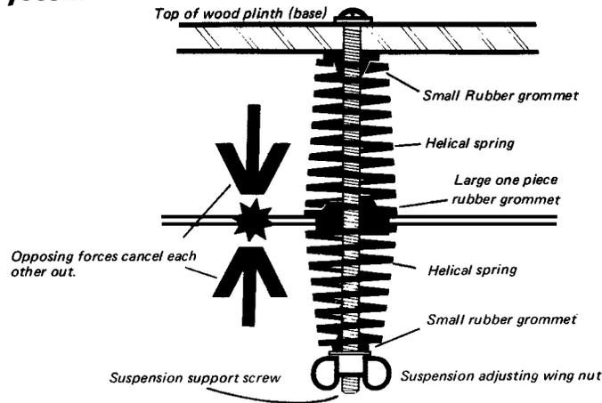
The arm mounting board is cantilevered from one arm of the T, and herein lies the one real problem I've had with the Fons. Supposedly the turntable and arm mount can be leveled by means of wing nuts on the three spring mounts. Well, one or the other, but not both at the same time. I finally resorted to shimming the arm board where it attached to the T, and after several hours achieved modest success in getting everything level.
